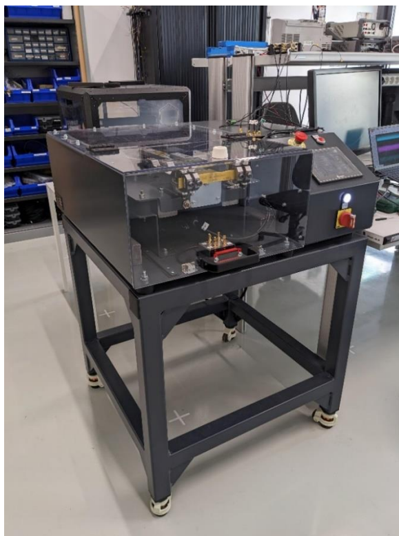
Figure 1 : Picture of the studied machine, designed to cyclically deform glass-fiber bars to study the fatigue life of Dragonfly® sensors.
